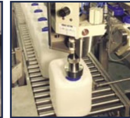
■ Exact positioning of a container in cap closing station
