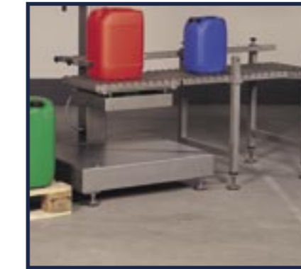
■ Non-driven container roller conveyor for semi-automatic system
