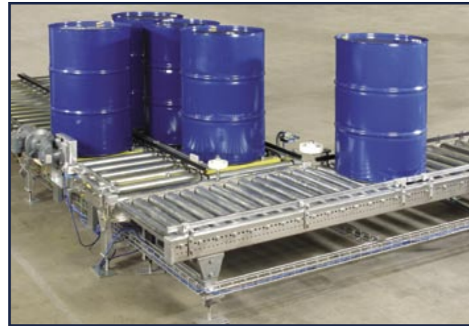
■ Empty drum in-feed via a dual roller conveyor with guide roller
