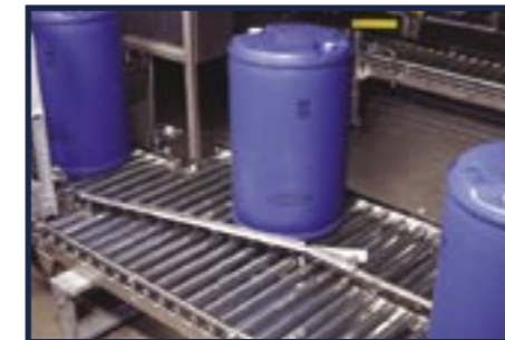
■ Filled drum feeding with pivoting diverter
