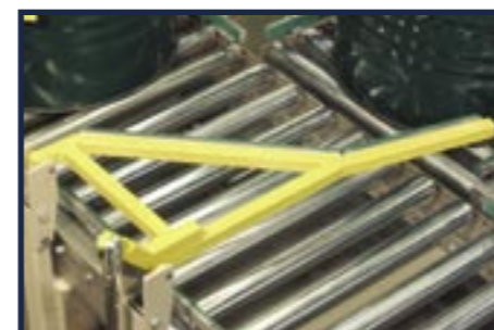
■ Guide for drum diversion
