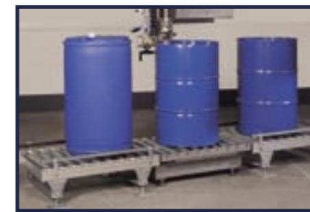
■ Non-driven drum roller for semi-automatic system
