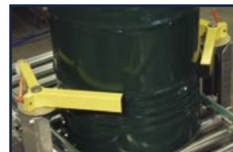
■ Separator for separating one drum from a row
